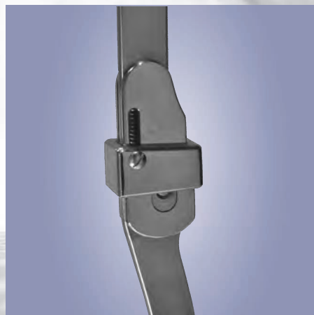
Internally housed spring automatically engages ring at full extension.
